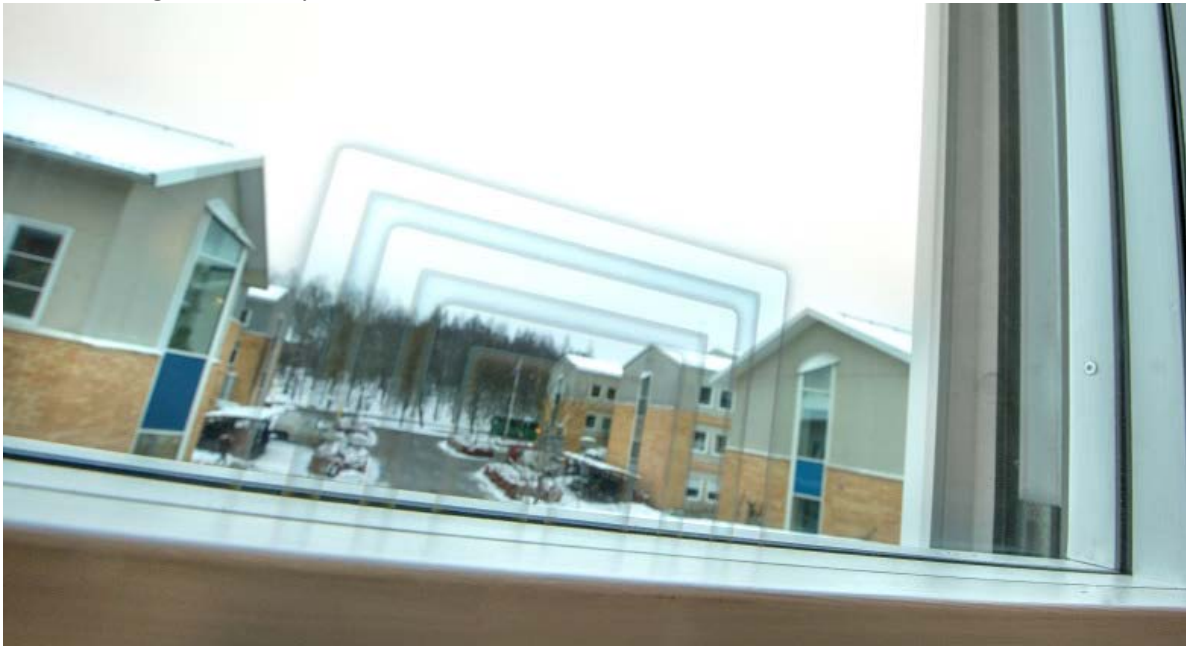
Figure 1. An example of Transparent Intelligence where a regular low energy coating on glass has been used to integrate a transparent antenna in a window.
