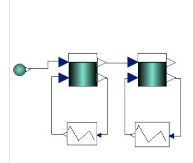
System model: Two connected tanks with controllers
