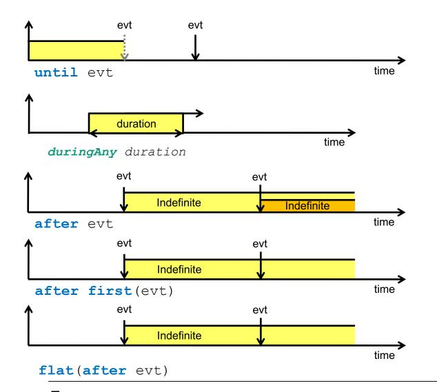
Special blocks that define when a requirement should be verified (after, until, afterFor...)
