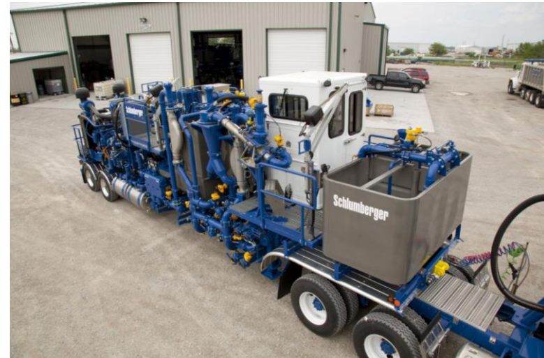
Cement additive metering system
