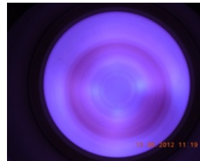
(a) Inductive mode ( B_s = 0 G), top view.
