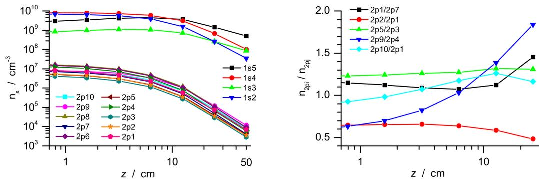
Figure 4: Left: Profiles of argon excited states densities obtained by the cr-model using the EEPF of figure 2 and further settings mentioned in the text. Right: Set of ratios of argon excited states densities.
