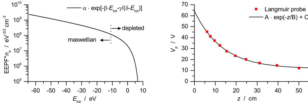
Figure 2: Models for the nonlocal EEPF (left) and for the profile of the plasma potential  $V_p$  (right) on the  $z$ -axis based on Langmuir probe data for a particular APS setting.  $\{\alpha, \beta, \gamma, \delta\}$ ,  $\{A, B, C\}$  are fitting parameters.
