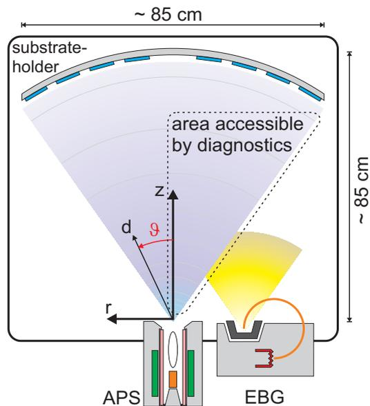
Figure 1: Scheme of the PIAD setup with plasma source (APS) and electron beam evaporator (EBG) at the bottom. The plasma diagnostics are positioned in the chamber by employing manipulators not shown in this figure. Note the indicated coordinate system.
