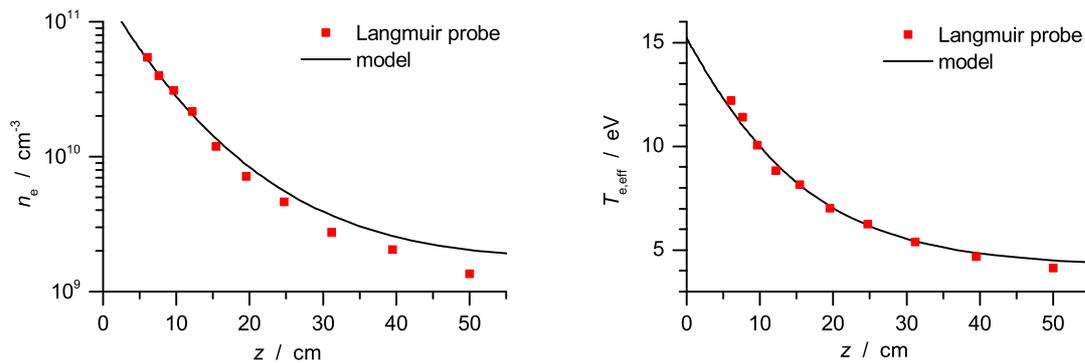
Figure 3: Electron density  $n_e$  (left) and effective electron temperature  $T_{e,eff}$  (right) as determined by the Langmuir probe and the trends according to the models shown in figure 2.
