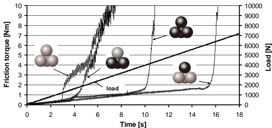
Fig. 2. Friction torque curves for various tribosystems.
