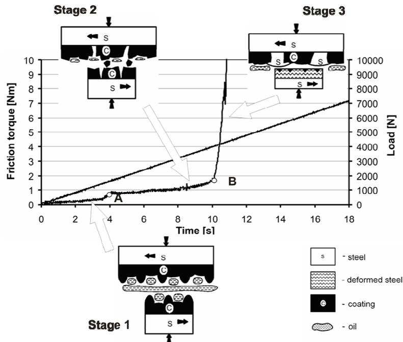
Fig. 3. The scuffing propagation in coating/coating tribosystem.
