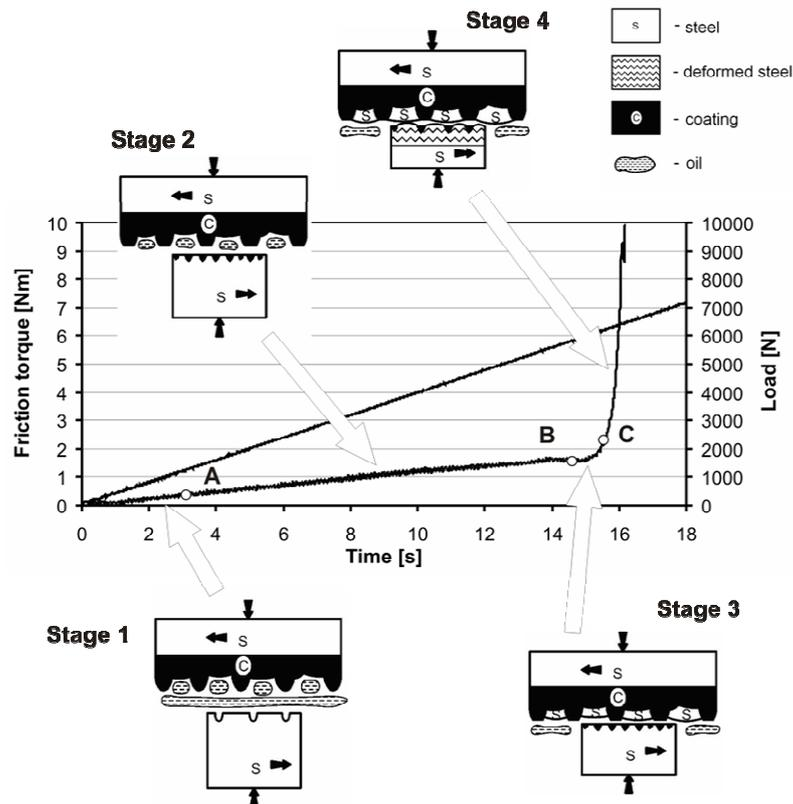
Fig. 4. The scuffing propagation in coating/steel tribosystem.
