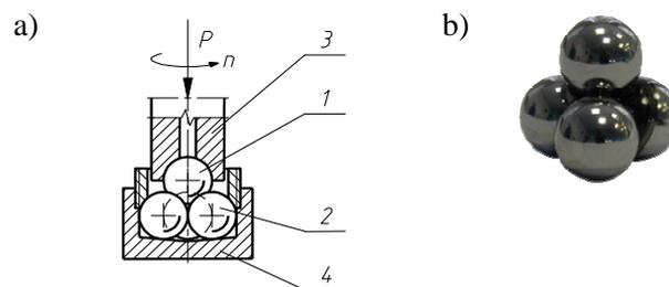
Fig. 1. Model four-ball tribosystem for testing scuffing: a) tribosystem: 1 - top ball, 2 - lower balls, 3- ball chuck, 4 - ball pot, b) photograph.
