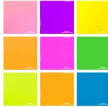
**Fig. 1:** Colour appearance of a Fabry-Perot stack ( $\text{SiO}_2\text{-Cr-SiO}_2$  on Al) with tilt effect; dependence on AOI and design features: normal incidence (upper line), AOI = 45° (centre line) and AOI = 60° (lower line); design A (left column), design B (centre column), design C (right column)
