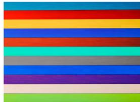
**Fig. 2:** Colour appearance of Fabry-Perot stacks without any tilt effect (Aradierung<sup>®</sup>)
