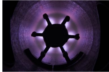
Photo 1 Cross-sectional view of plasmas for multiple units wire stripper.
