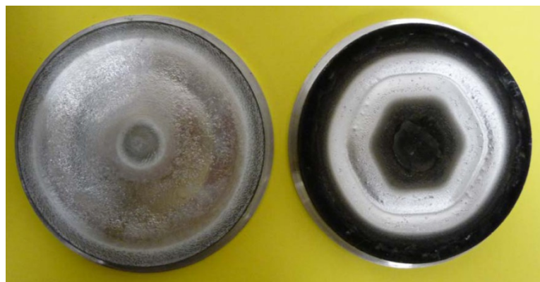
Fig. 1 View of the Al targets exploited in the GIMS (left photo) and under the condition of continuous working gas flow (right photo), respectively in the nitrogen only and Ar+N 2 atmosphere.
