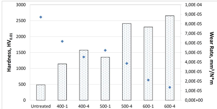
Fig. 2. Microhardness values of untreated and nitrided specimens
