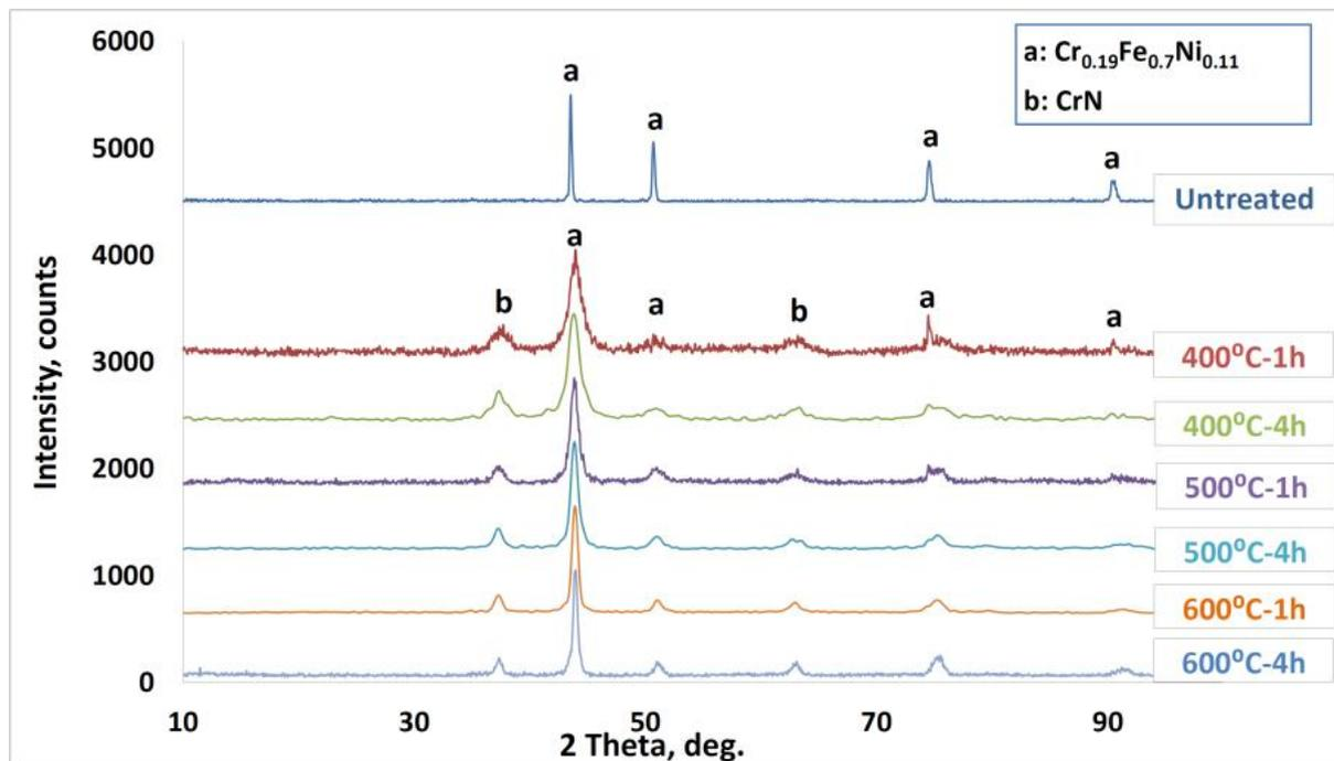
Fig. 1. XRD patterns of specimens
