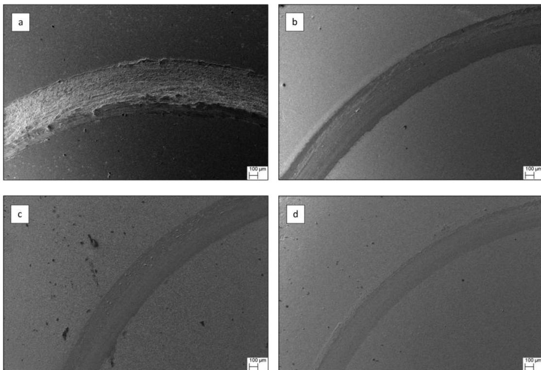
**Fig. 5.** SEM images obtained from different nitriding conditions; untreated specimen (a), 400-4 (b), 500-4 (c), 600-4 (d)
