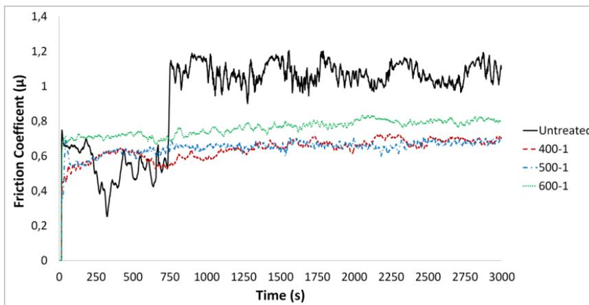
Fig. 3. The change of friction coefficient versus time at 1 h and different temperatures
