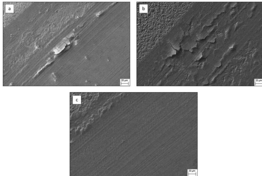
**Fig. 6.** Detailed SEM images obtained from different nitriding conditions; 400-4 (a), 500-4 (b), 600-4 (c)
