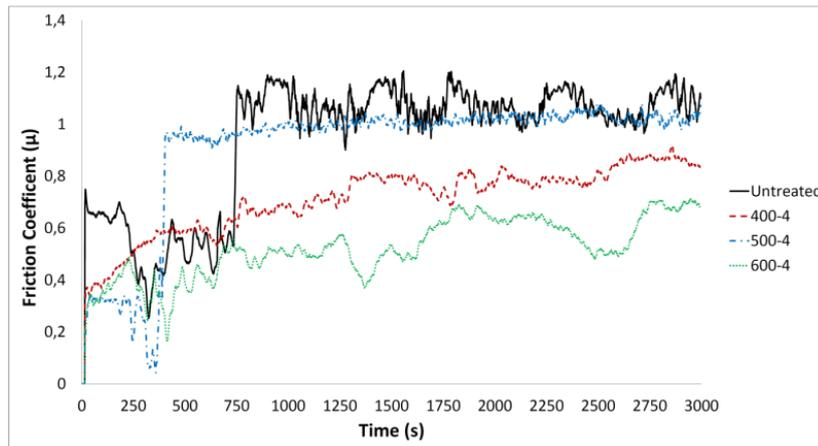
**Fig. 4.** The change of friction coefficient versus time at 4 h and different temperatures
