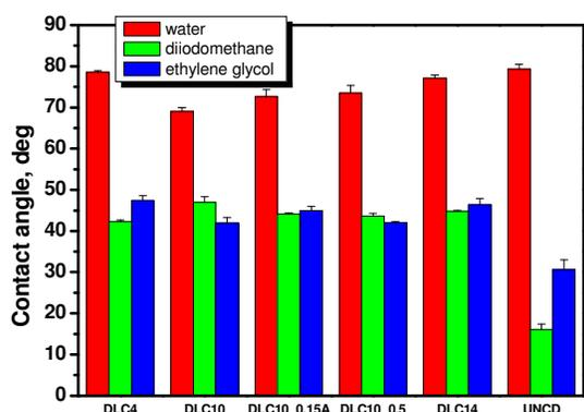
**Figure 2:** Wettability of DLC and UNCD films with water, diiodomethane and ethylene glycol
