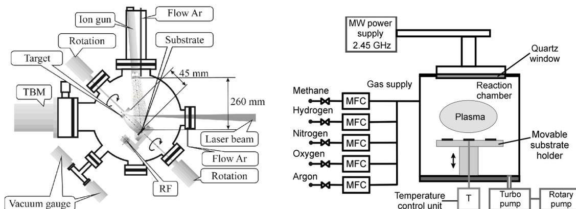
**Figure 1:** Scheme of PLD deposition system with ion bombardment (left) and MWCVD (right)
