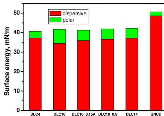
**Figure 3:** Total surface energy  $\gamma$  of DLC and UNCD films shown with dispersive  $\gamma^d$  and polar  $\gamma^p$  components
