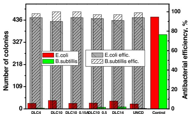
**Figure 4:** Number of *E. coli* and *B. subtilis* colonies on DLC and UNCD films and the respective antibacterial efficiency
