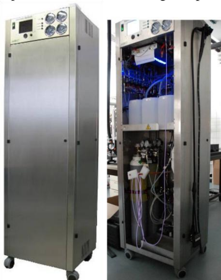
Figure 9: Demonstrator for a reprocessing unit for endoscopes equipped with bifilar plasma generator
