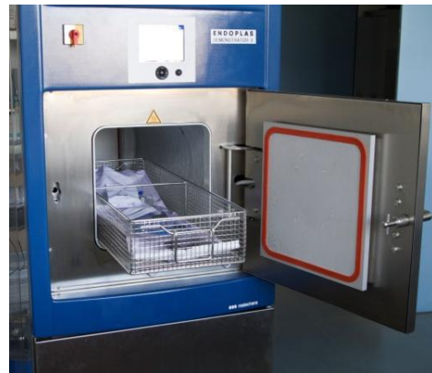
Figure 4: commercial sterilizer with integrated PLeXc ® plasma source
