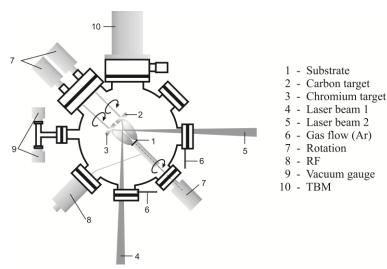
Figure 1 The scheme of dual PLD deposition system
