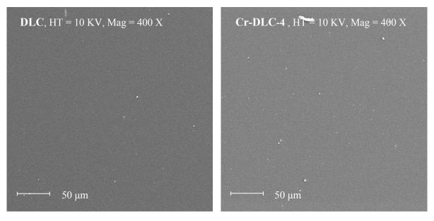
Figure 2 SEM micrographs showing surface DLC and Cr-DLC-4
