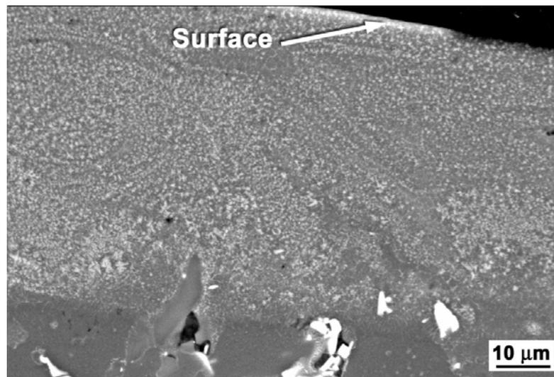
Fig. 3 Cross-section morphology of the Ti (2.5  $\mu\text{m}$ ) /silumin system sample after CPF treatment with the energy density of  $19 \text{ J/cm}^2$  (e).
