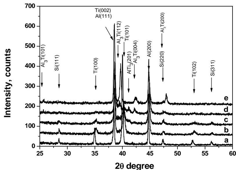
Fig. 1 XRD diffraction patterns of the Ti (2.5  $\mu\text{m}$ ) /silumin system samples before (a) and after CPF treatment with the energy density of  $4 \text{ J/cm}^2$  (b),  $7 \text{ J/cm}^2$  (c),  $13 \text{ J/cm}^2$  (d),  $19 \text{ J/cm}^2$  (e).
