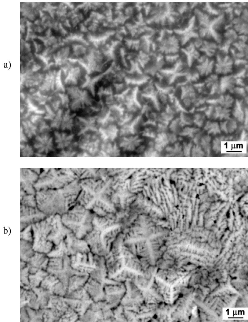
Fig. 4 Cross-section morphology of the Ti (2.5  $\mu\text{m}$ ) /silumin system (a) and Ti (5.5  $\mu\text{m}$ ) /silumin system samples after CPF treatment with the energy density of  $19 \text{ J/cm}^2$  (a) and  $7 \text{ J/cm}^2$  (b).
