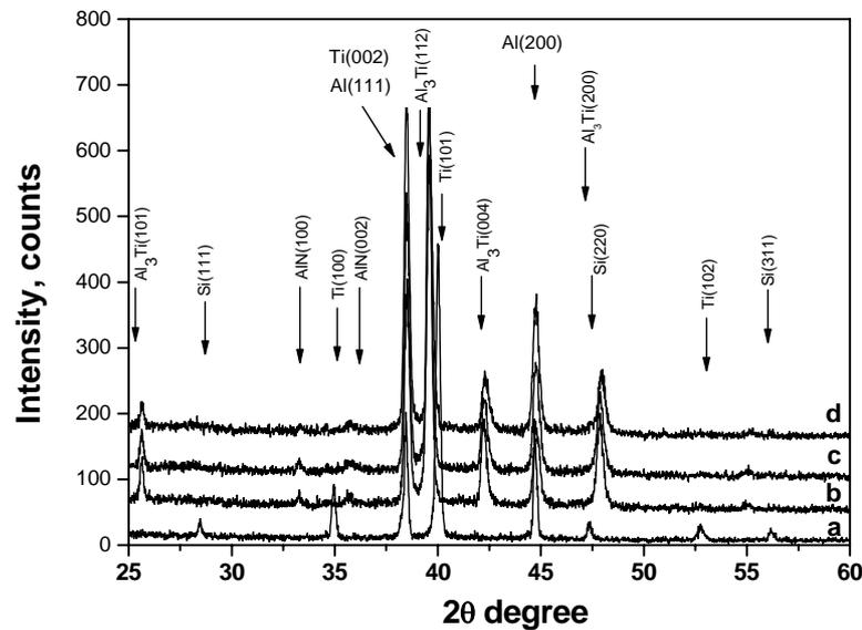
Fig. 2 XRD diffraction patterns of the Ti (5.5  $\mu\text{m}$ ) /silumin system samples before (a) and after CPF treatment with the energy density of  $7 \text{ J/cm}^2$  (b),  $13 \text{ J/cm}^2$  (c),  $19 \text{ J/cm}^2$  (d).
