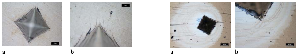
Fig. 8. Defects of the TiN coating on the SW7M (1.3343) steel around the indentation after the HV5 hardness test: a - fractures and micro-chipping of the TiN coating on the indentation edge, b - coating fractures propagating in various directions
