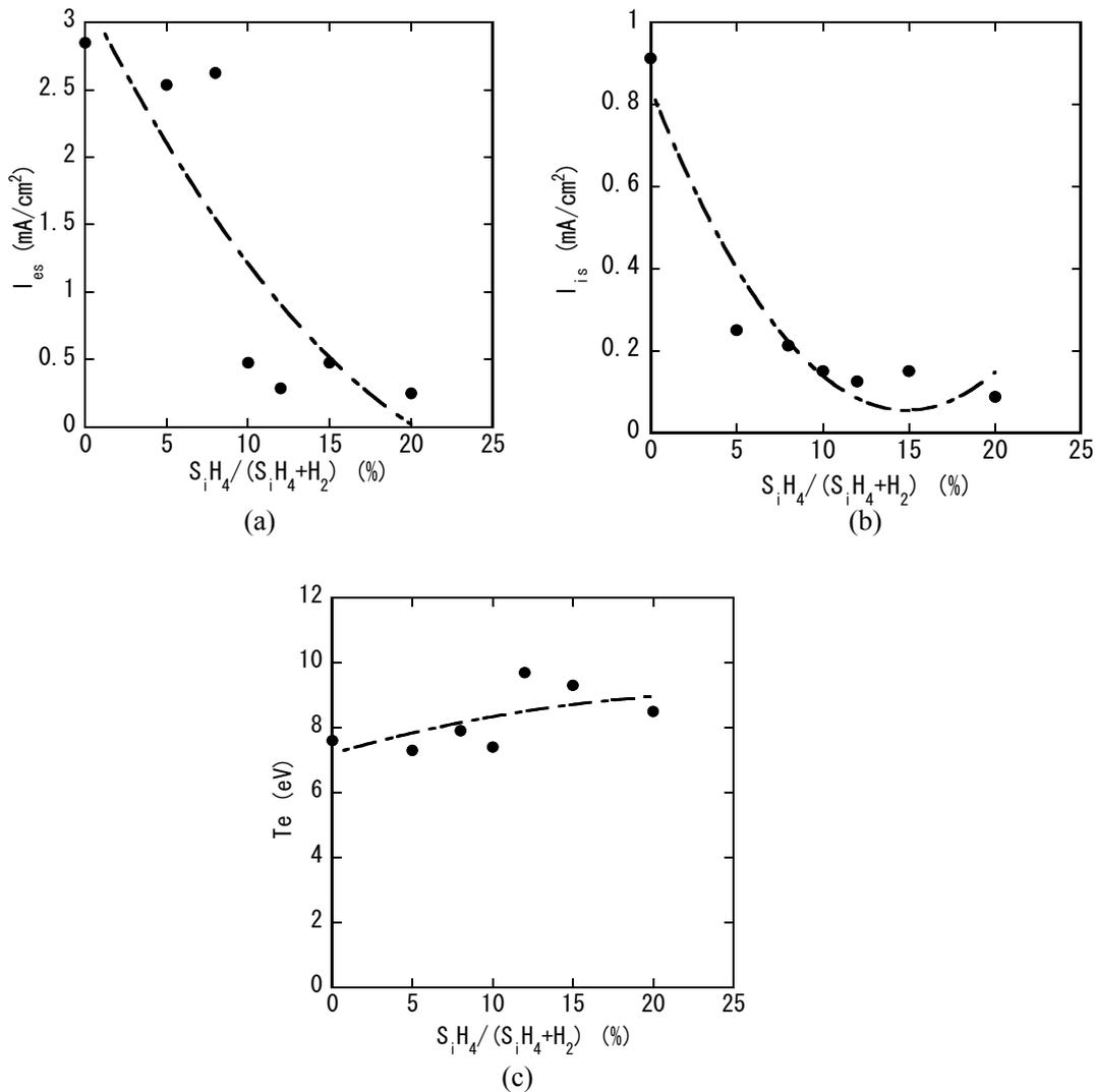
Fig. 1 Plasma parameter measurements: (a) the electron saturation current, (b) the ion saturation current and (c) the electron temperature.
