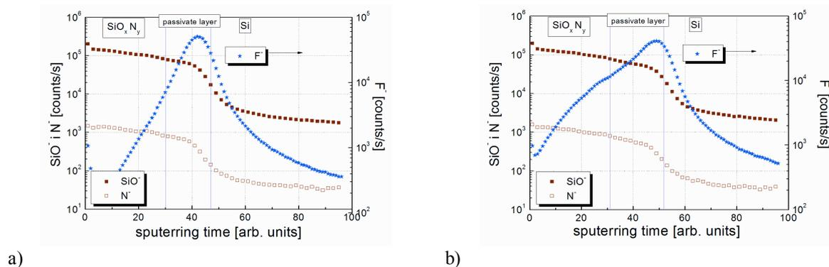
Fig. 1 Comparison of SiO<sup>-</sup>, N<sup>-</sup> and F<sup>-</sup> profiles within the silicon oxynitride layers after modification of silicon substrate in PECVD (a) and RIE (b) reactor.
