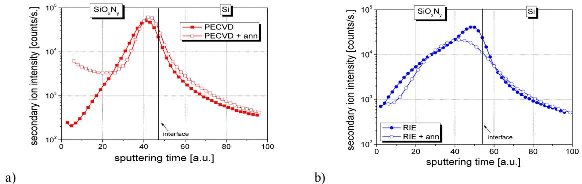
Fig. 2 Thermal stability of fluorine concentration within the SiO<sub>x</sub>N<sub>y</sub> layers after modification of silicon substrate in PECVD (a) and RIE (b) reactor.
