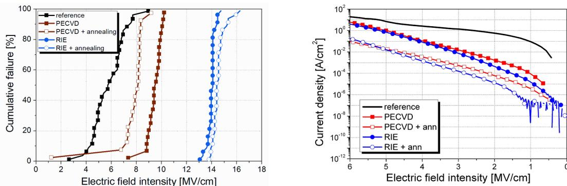
a) b) Fig. 5 Cumulative failure of a) MOS structures; b) MIS structures, investigated in the course of this work
