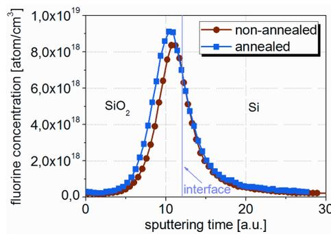
Fig. 3 Thermal stability of fluorine concentration within the  $\text{SiO}_2$  layer after modification of silicon substrate.
