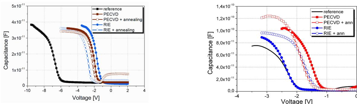
a) b) Fig. 4a Comparison of C-V characteristics of a) MOS structures; b) MIS structures, fabricated on modified silicon substrates; C-V characteristics of reference structure was also shown.
