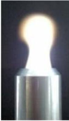
Figure 1: microwave excited plasmasource PLeXc® developed by INP
