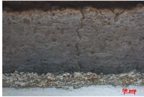
Fig.2. After corrosion testing, micrograph of sample 3
