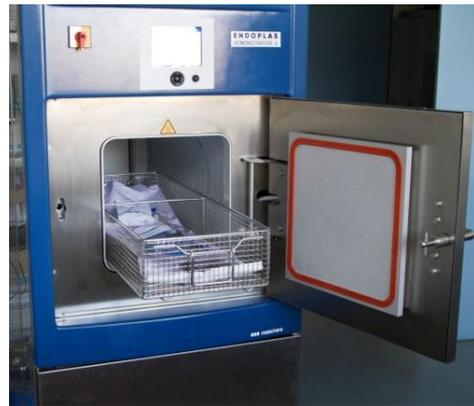
Figure 4: commercial sterilizer with integrated PLeXc® plasma source
