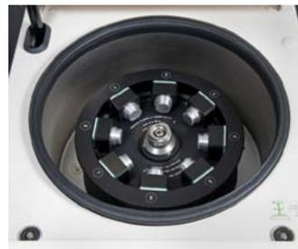
Fig. 2: Drum rotor equipped with eight testing units
