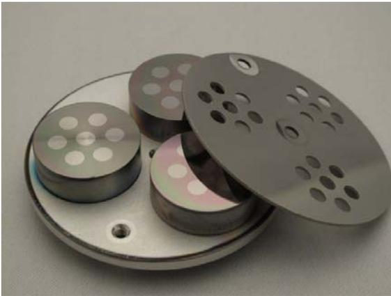
Fig. 1: Samples with spot mask for conducting layer
