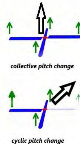
Fig. 3 Collective and cyclic pitch.
