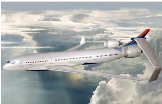
Fig. 1 Joined-wing aircraft concept of "the future". [2]
