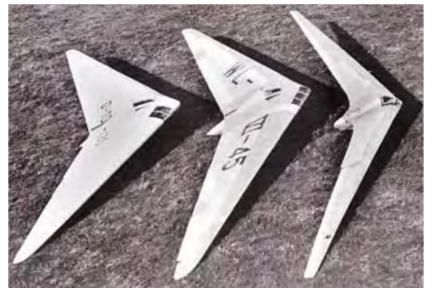
Fig. 2 The Horten Ho 2, 3 and 4 Gliders. Courtesy: Nickel and Wohlfahrt [2]
