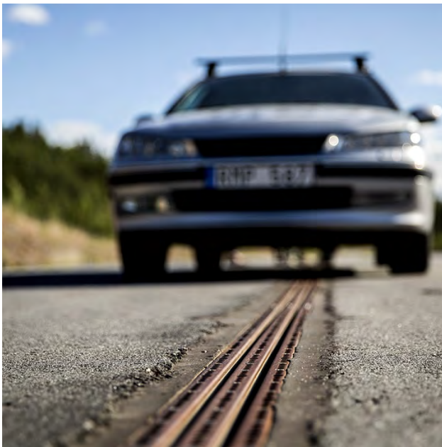
Fig. 2 Conductive Power Transfer(In-road Rail) for Electric Vehicle[6].
