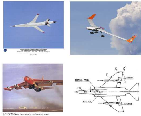
Fig. 4 . few of the testbeds used for Active flutter suppression system (from top)NASA DAST,Lockheed X56,B-52 and F404
