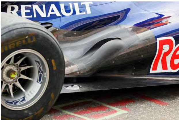
Fig. 2 . Red Bull RB8 Coandă exhaust.
