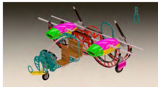
Fig. 2 . Fuselage and center section structure (gas powered version), 2013
