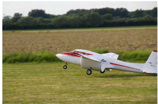
Fig. 8 . Landing at high angle of attack
