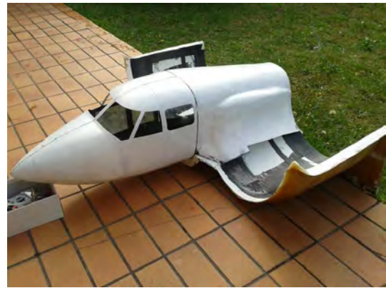
Fig. 4 . composite parts. Carbon reinforcement for the "channel" spar, leading and trailing edge and in the fuselage nose to transmit the forces from the nose gear , 2014
