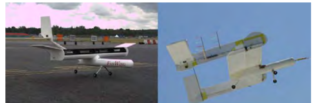
Fig. 2 . FanWing prototypes: 2008 version (left) and 2011 version (right) [3]
