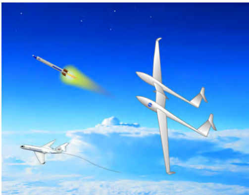
Fig. 1 Illustration of towed glider air-launch system.[3]
