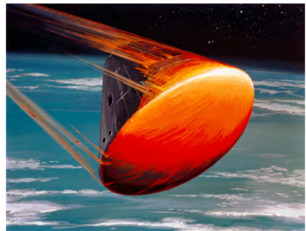
Fig. 3 A blunt nosed re-entry module entering the atmosphere illustrating the temperature difference along the surface [8].
