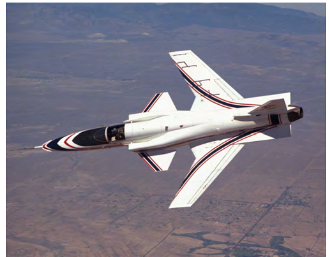
Fig. 2 The experimental aircraft Grumman X-29 and its forward swept wings.[3]
