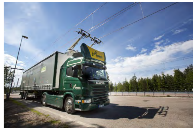
Fig. 1 Conductive Power Transfer(Overhead) for Electric Vehicle[4]
