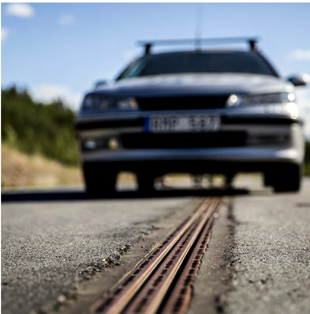
Fig. 2 Conductive Power Transfer(In-road Rail) for Electric Vehicle[6].
