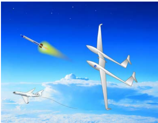
Fig. 1 Illustration of towed glider air-launch system.[3]
