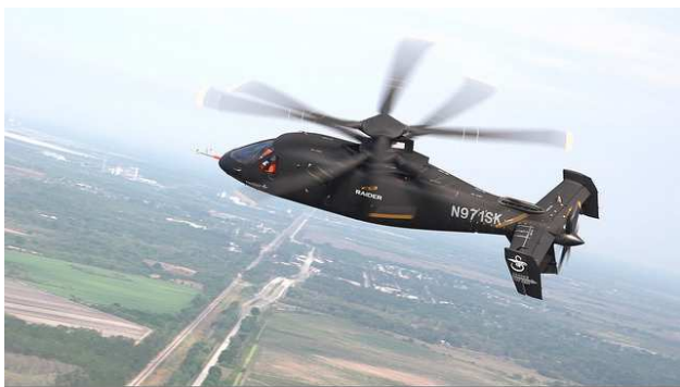
Fig. 1 . Picture of the Sikorsky S-97 Raider. Utilizing a coaxial main rotor and an aft propeller as well as retractable landing gears. Photo courtesy Lockheed Martin
