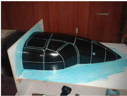
Fig. 3 . Nose section master ready for the mold manufacturing, December 2013
