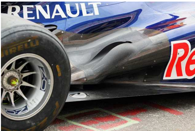
Fig. 2 . Red Bull RB8 Coandă exhaust.
